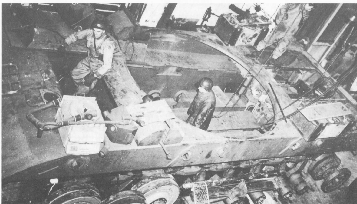
Left: The partially assembled E-100 chassis as found by Allied troops at a Henschel facility near Paderborn in March 1945. (NA)
