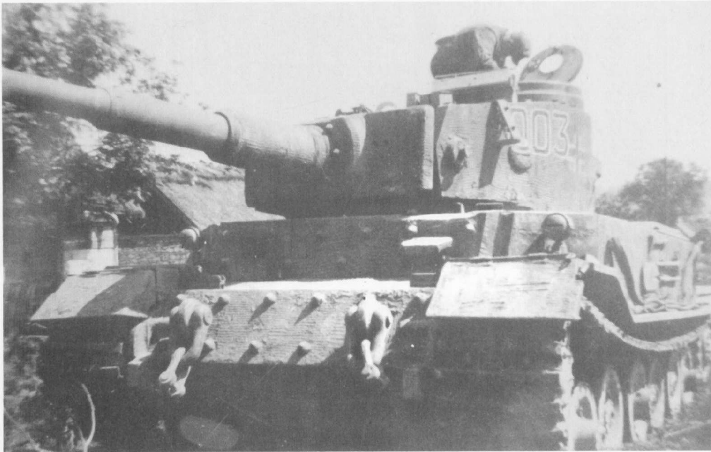
Left and Below: The only Panzerkampfwagen VI P known to have been used in combat was completed by Nibelungenwerk as a Panzerbefehlswagen (Fgst.Nr.150013) with a new turret with higher roof (Krupp Turm Nr.14). (KHM)
