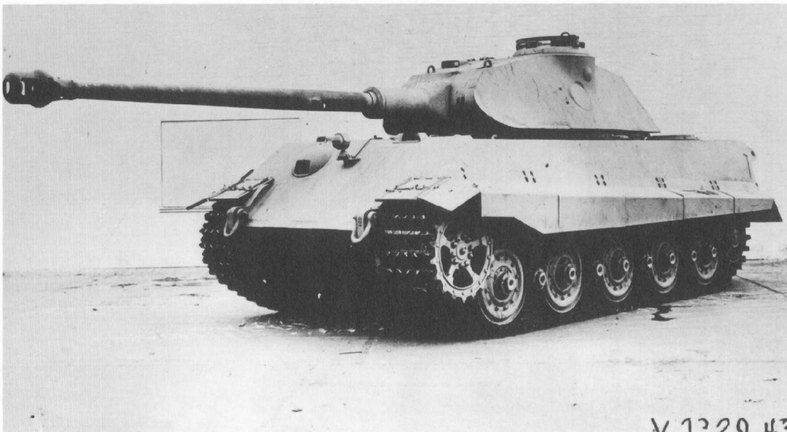
Left: The first Tiger II (Fgst.Nr.V1) completed by Henschel in November 1943 with the Krupp turret designed for the Porsche Typ 180. The turret had 25-mm-thick fore and aft roof plates. (WJS)
