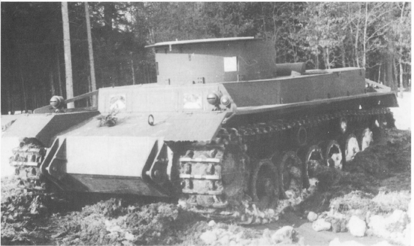
Above and Below: A concrete test weight was mounted in place of a turret on the Porsche Typ 100 chassis with “soft” steel hull. The turret with an 8.8 cm Kw.K. L/56 gun, designed by Krupp for mounting on the Porsche Typ 100, was used for the Porsche Typ 101 and Henschel Tiger I. (WJS)
