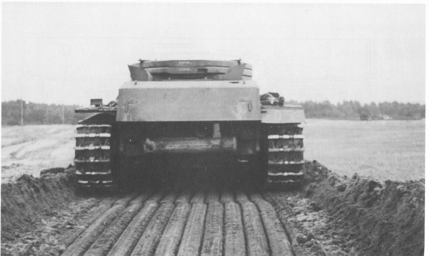
Above and Below: The VK 30.01 (H) Versuchsfahrgestell (Fgst.Nr.2) being used to test trench-digging equipment at Haustenbeck on 30 January 1944. It was the second chassis assembled by Henschel from a trial series of three. (WJS)
