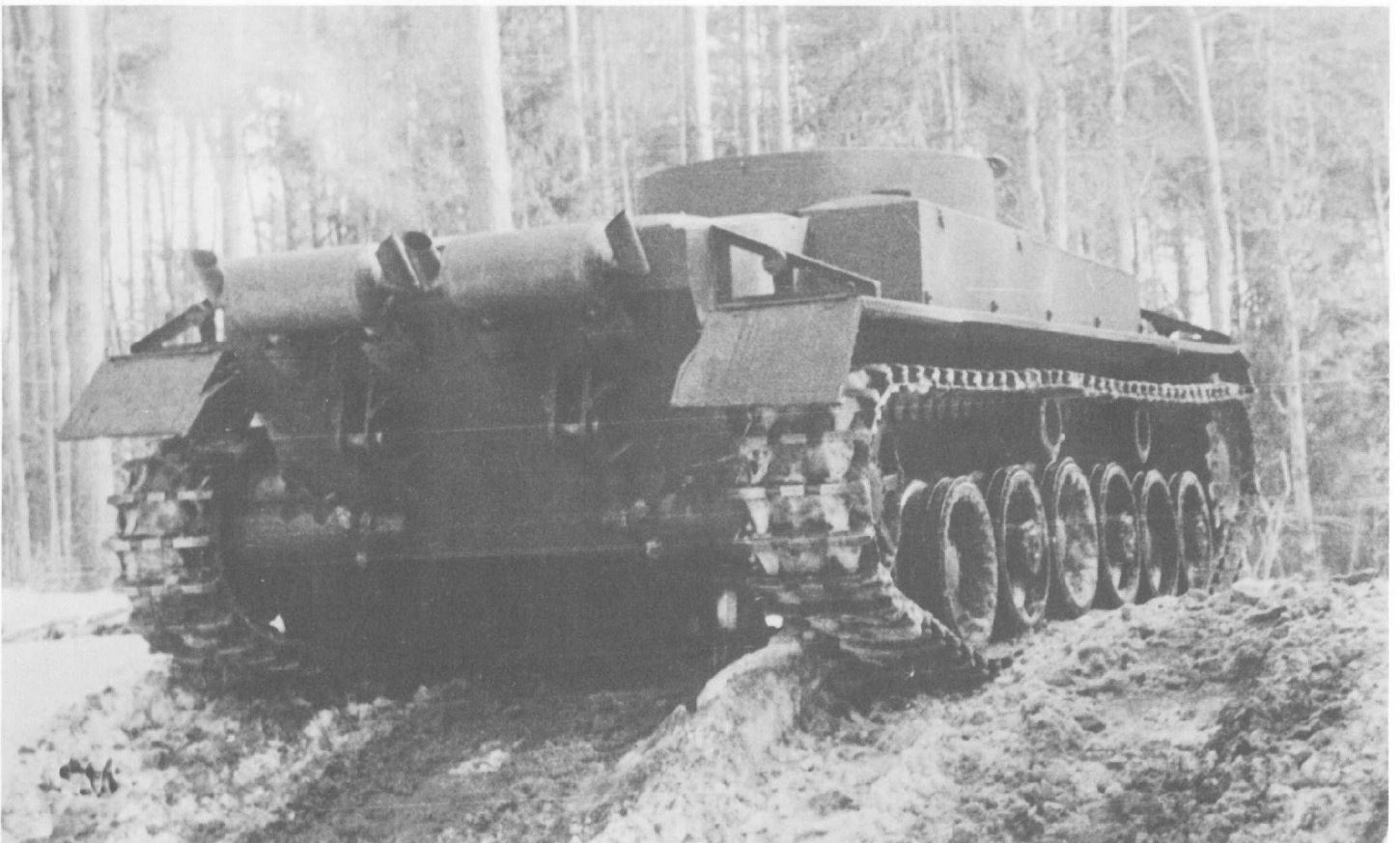
Above and Below: A concrete test weight was mounted in place of a turret on the Porsche Typ 100 chassis with “soft” steel hull. The turret with an 8.8 cm Kw.K. L/56 gun, designed by Krupp for mounting on the Porsche Typ 100, was used for the Porsche Typ 101 and Henschel Tiger I. (WJS)
