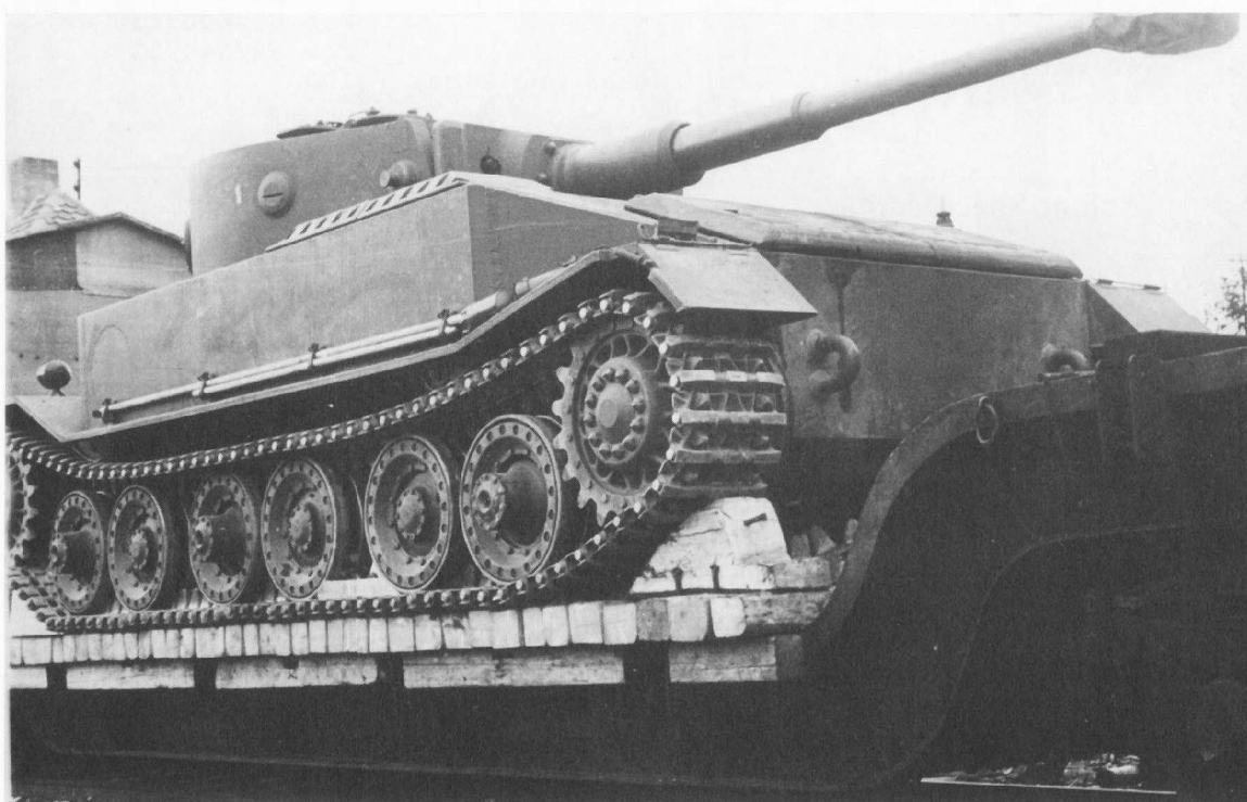
Left: The first VK 45.01 (P) completed at Nibelungenwerk being shipped by rail for demonstration to Hitler on 20 April 1942. It has Krupp turret Nr.1 but it wasn't chassis number 1. (WJS)
