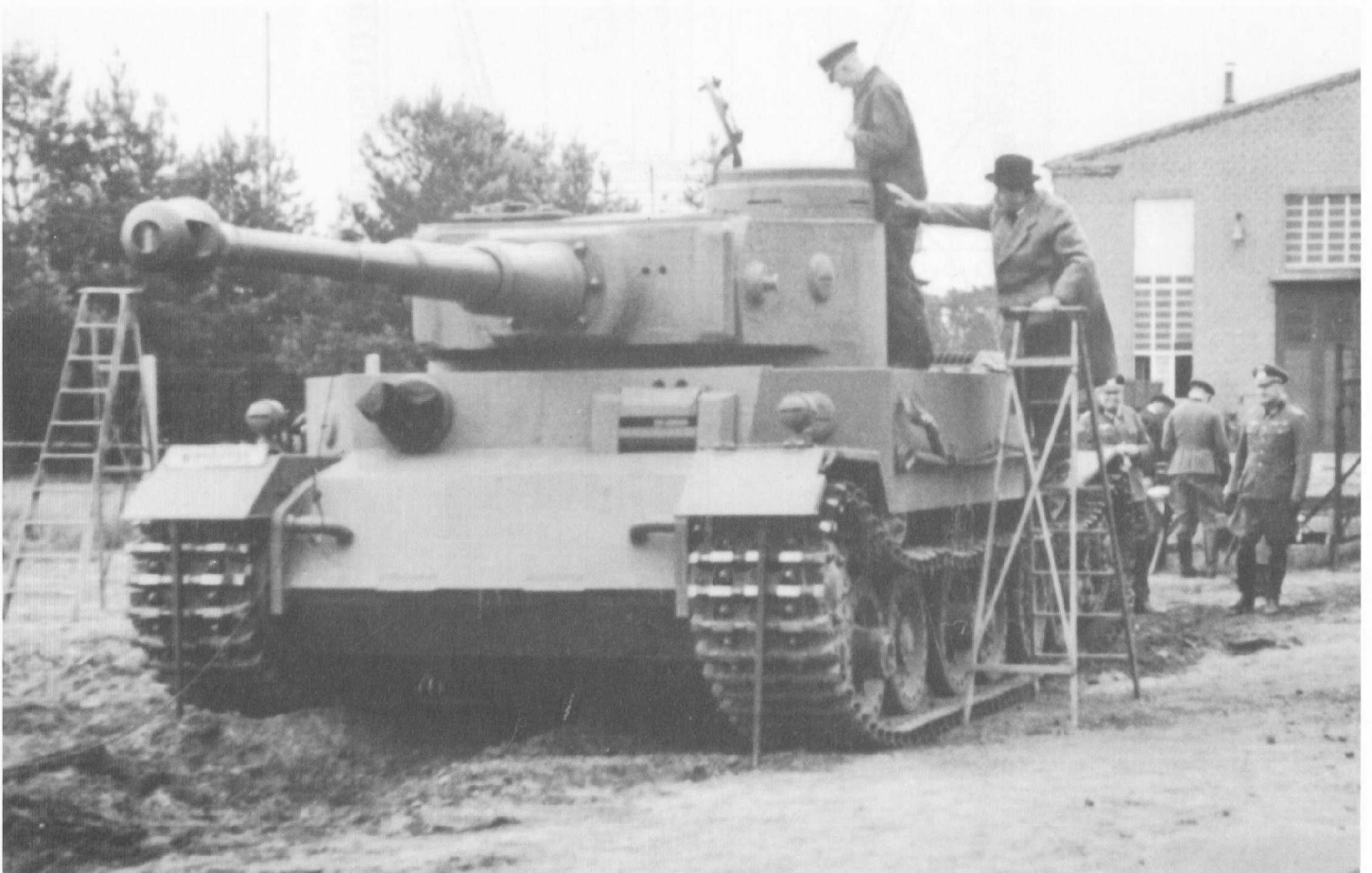
This and Opposite Page: The second Panzerkampfwagen VI (P1), completed at Nibelungenwerk in June 1942 with Krupp Turm Nr.3, is being inspected by Dr. Porsche. (Porsche)
