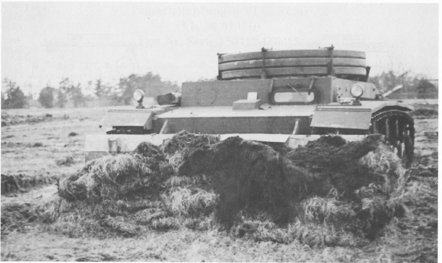
Above and Below: The VK 30.01 (H) Versuchsfahrgestell (Fgst.Nr.2) being used to test trench-digging equipment at Haustenbeck on 30 January 1944. It was the second chassis assembled by Henschel from a trial series of three. (WJS)
